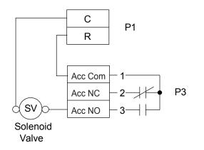
**Figure 9b: Open Loop Solenoid Valve Connection Option** Typical slow operating external 24V water solenoid valve (type VM) wiring.
